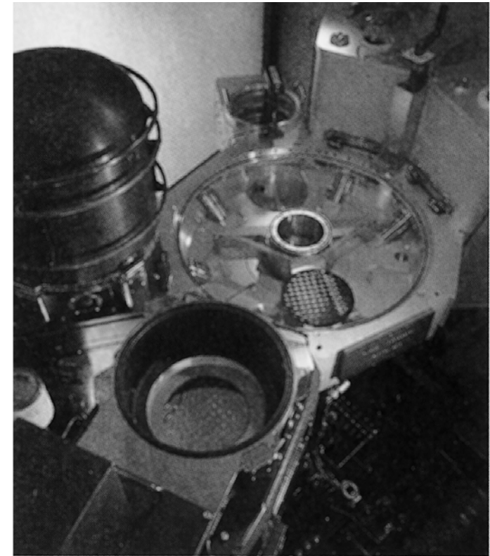
Figure 11.21 Applied Materials high-density plasma silicon etch system (photo courtesy Applied Materials).
